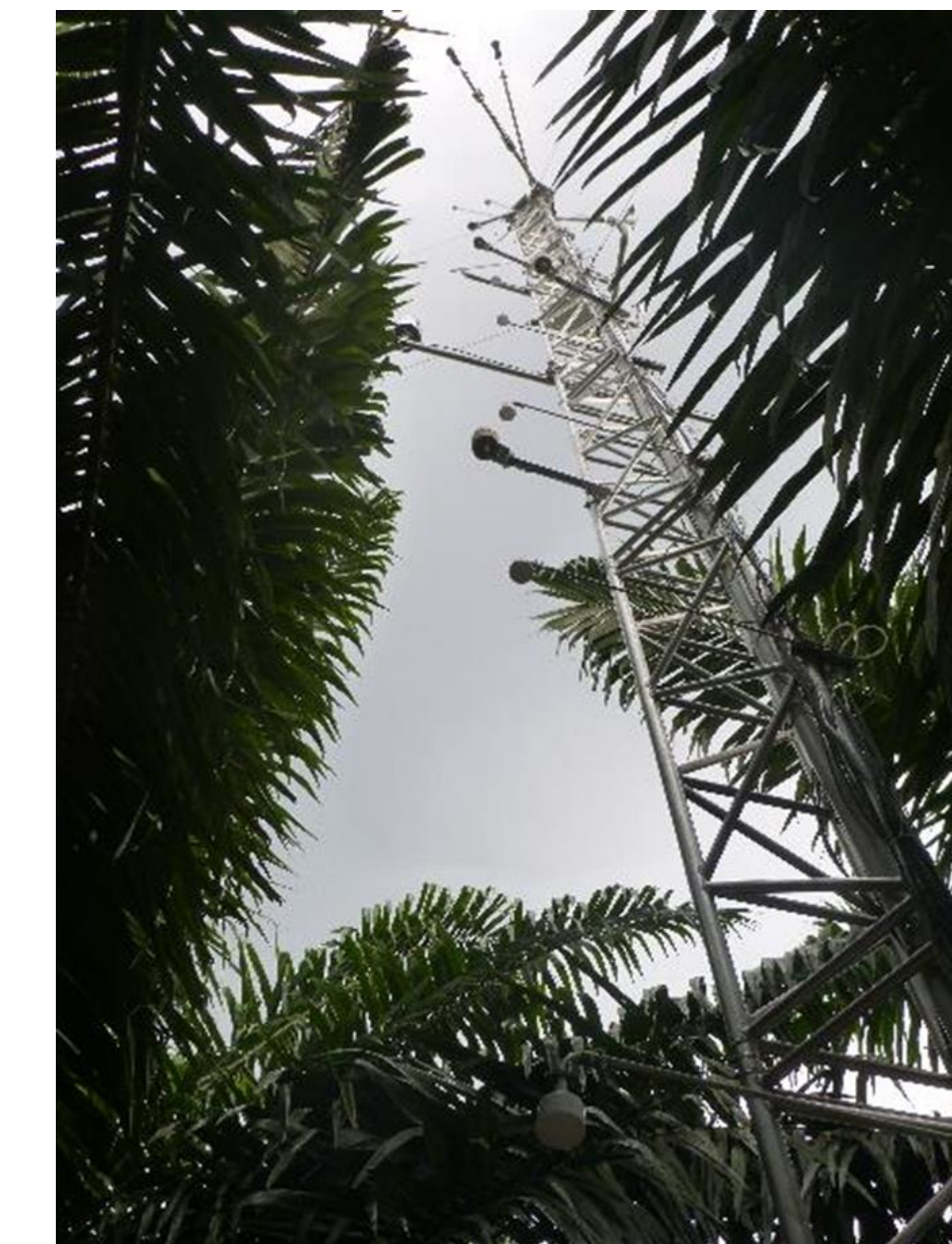
12-yr old: 22 m tower CO 2 , H 2 O and CH 4 (Licor 7500A and FGGA, Los Gatos)
